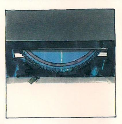
However, if a line splits the bottom of the image as shown, roll the control to the left (when facing the screen) until the line disappears. If the image is split on top, roll the control to the right.
